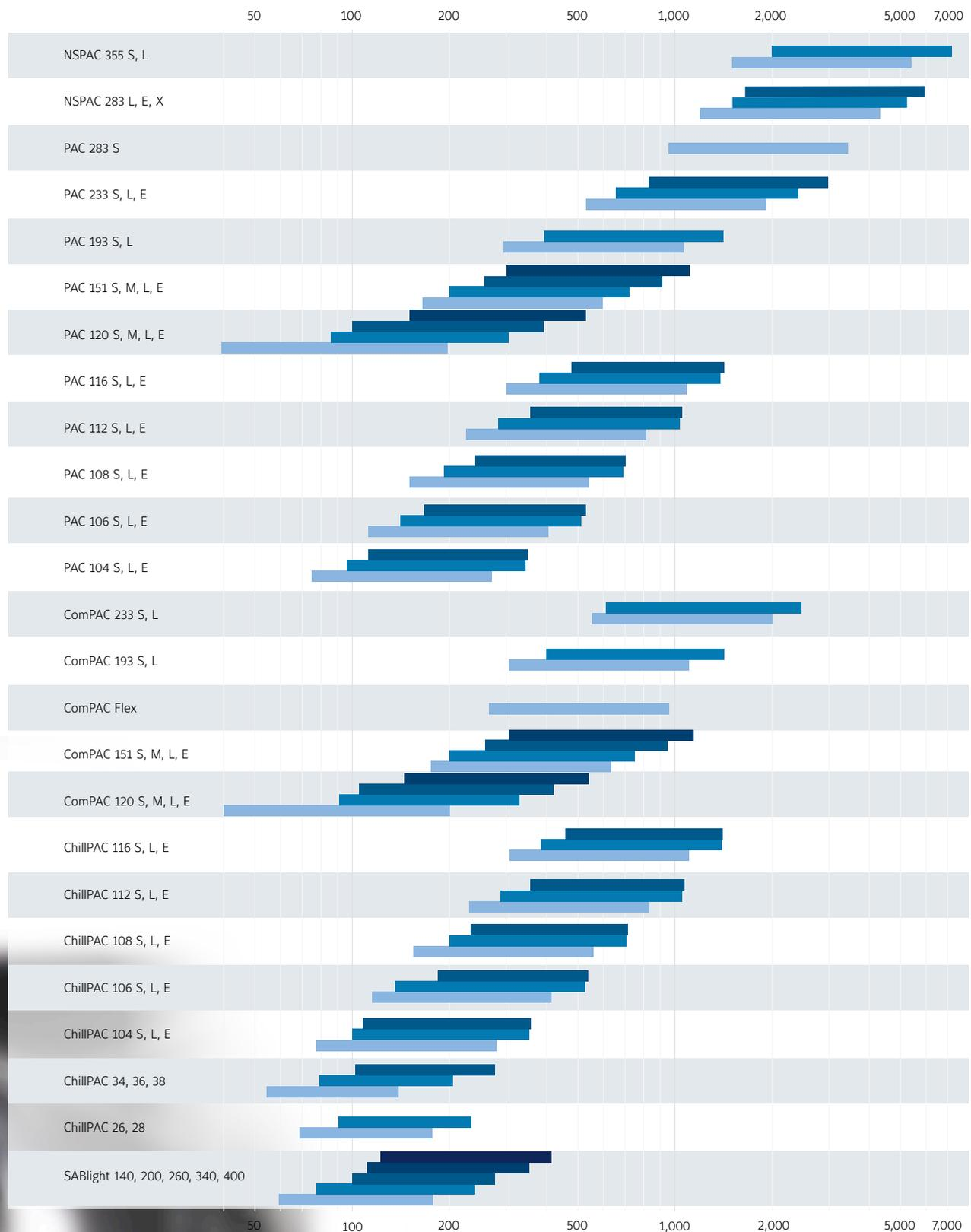
Capacities in kW at 7/12°C (cold side) and 30/35°C (hot side) in maximum speed (Reciprocating compressors at 50/60 Hz. Screw compressors at 50/60/70/100 Hz)
